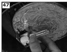
Install 1 x 100 halogen bulb E-11. Do not touch bulb surface as oily residue from skin can cause the bulb to explode.
